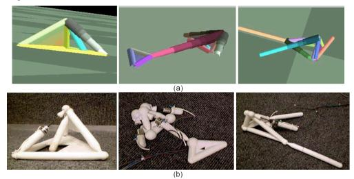
Figure 2: Evolving bodies and brains: (a) Three evolved robots, in simulation (b) the three robots reproduced in physical reality using rapid prototyping. From [6].
