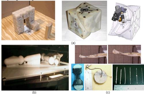
Figure 4: Transferring morphological changes into reality (a) Reconfigurable *molecube* robots [14], (b) Rapid prototyping, (c) Future rapid prototyping systems will allow deposition of multiple integrated materials, such as elastomers, conductive wires, batteries and actuators, offering evolution a larger design space of integrated structures, actuators and sensors, not unlike biological tissue. From [7].
