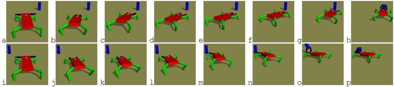
Fig. 7. A sample successful controller for **robot 2**. **a-h**: The robot moves toward the target object placed 3.9 meters ahead and to the right while turning (**a-d**), turns too far (**e,f**), compensates (**g**) and then picks up the target object (**h**). **i-p**: The robot moves toward the target object placed equal-distance away on the left side without overshooting (**i-n**) and swings it onto its back (**o-p**).
