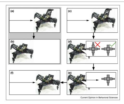
Robot prospection. A robot incapable of prospection (a) is unable to move once it suffers physical damage, such as the loss of part of a leg (b). Another robot that can move and can predict (c), once damaged, mentally simulates its situation and deduces that it has been damaged (d). It then mentally rehearses a motor program that will enable it to regain the ability to move despite its injury (e). Finally, it executes that motor program and thus autonomous recovers from the injury (f).
