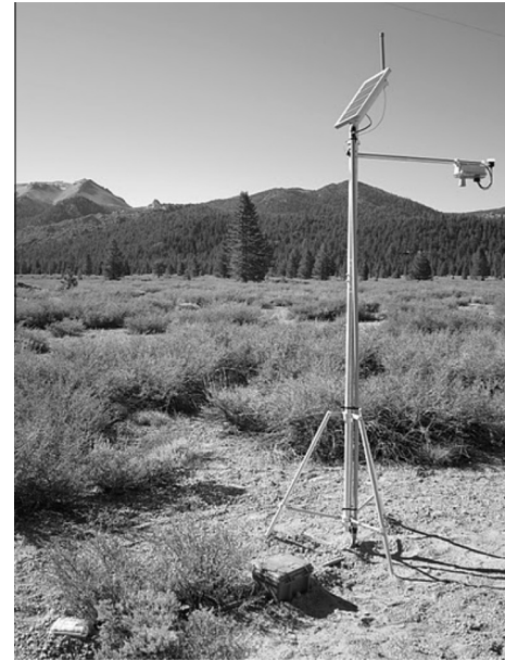
Fig. 3. Snowcloud WSN sensor tower. A complete sensor stand with solar-recharged battery power, wireless mesh communication, and multiple sensor modalities. October 2011, Mammoth Lake, CA.
